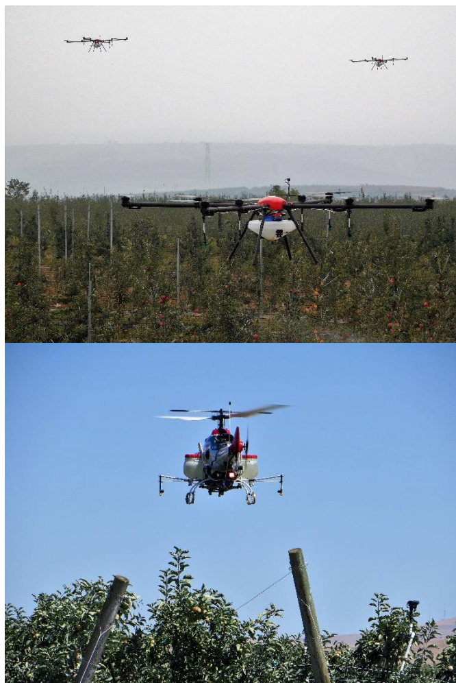
Figure 1. Small- (top) and mid-sized (bottom) UAS being tested for orchard spraying application. (Photos by Lav Khot, WSU.)
