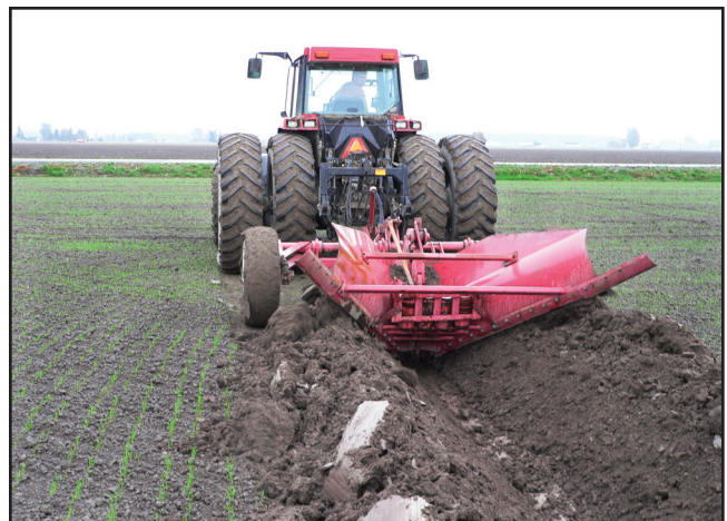
Figure 2. V-ditcher used to dig ditches through fields to improve drainage during winter rains. (Photo by Jonathan Roozen, Washington State University Extension)
